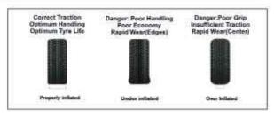
Tyre Pressure: Maintain recommended tyre pressure as mentioned below, to increase life of the tyre and for better fuel consumption.
